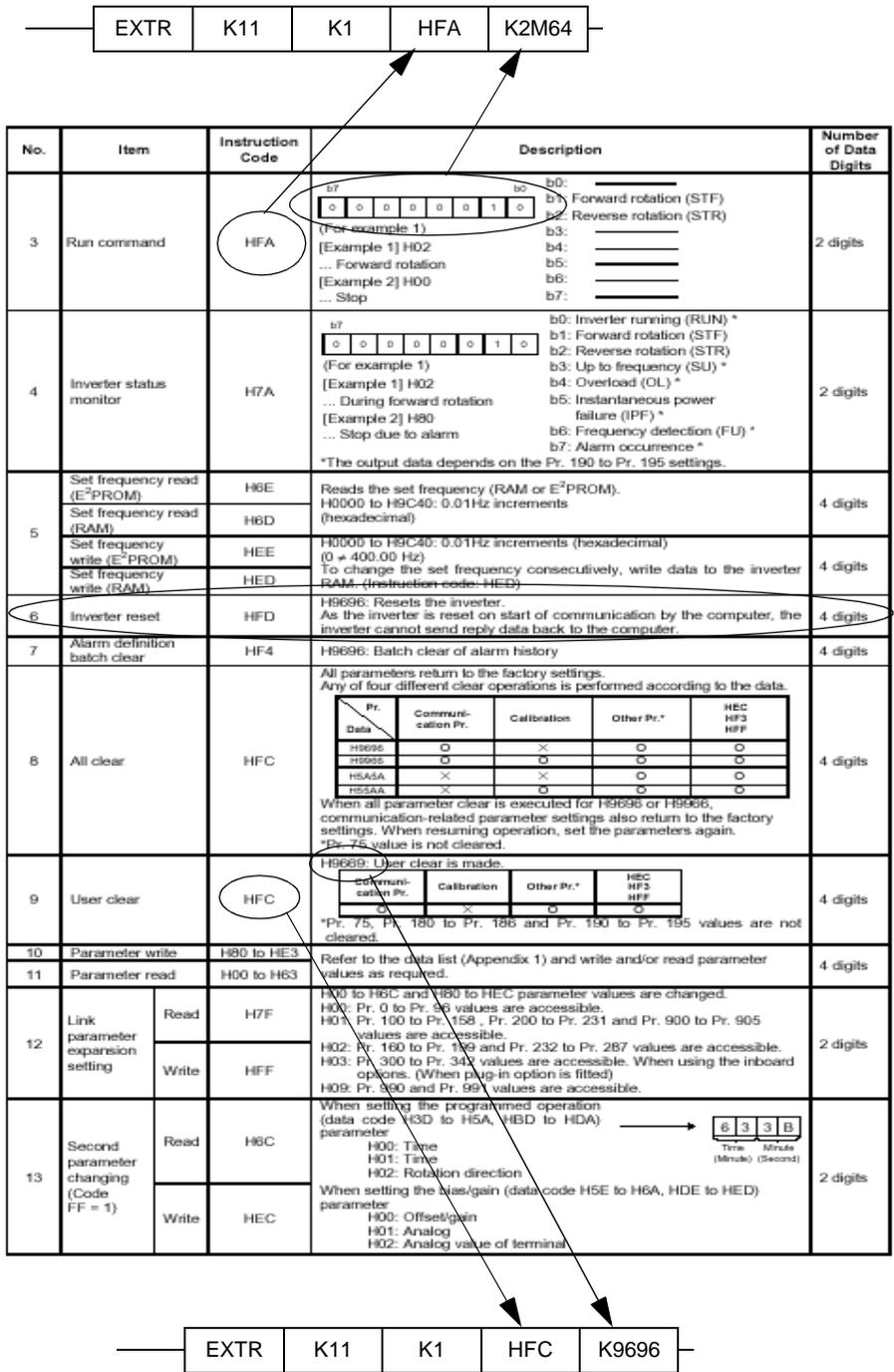
For 2 seconds after the reset instruction is transmitted, the inverter does not accept communication. As this period of time is controlled by the PLC, the sequence does not need to be taken into consideration
