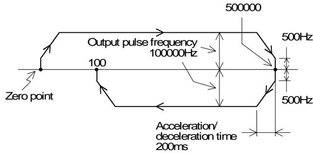
In this example the actual output frequency for the first step, acceleration, and the last step, deceleration, can be obtained using the following expression.
