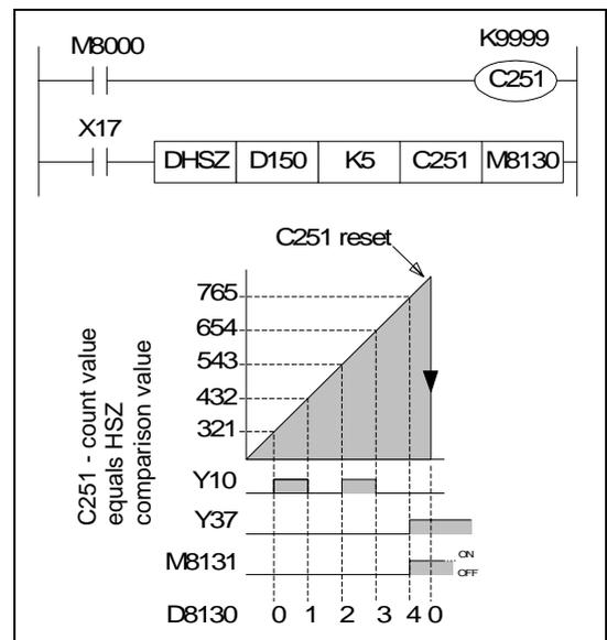
**Operation 3 - Combined HSZ and PLSY Operation:** (Applicable units: FX2N and FX2NC)
