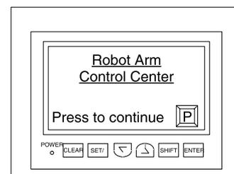
This example uses the IST instruction (FNC 60) to control the operation mode of the robot arm. The program shown opposite identifies how the IST instruction is written into the main program.
