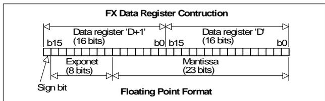
Valid ranges for floating point numbers as used in FX Main Processing Units:
