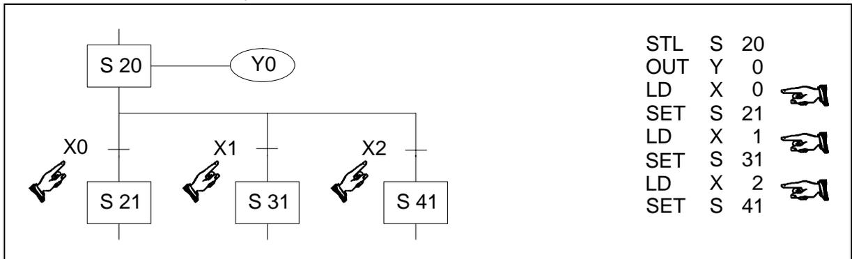
A programming construction to split the program flow between different branches is very useful but it would be more useful if it could be used with a method to rejoin a set of individual branches.
