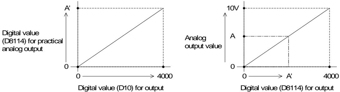
Because A is smaller than 10 Volts, the digital value of 0~4000 must be converted to a value of 0~A' as shown in the graphs above.  $4000/10V = A'/A$  or  $A' = [4000/10] \times A = 400 \times A$
