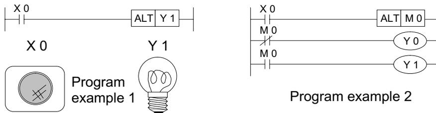
Pressing the momentary push button X1 once will switch the lamp ON. Pressing the push button for a second time will cause the lamp to turn OFF. And if the push button is again pressed for a third time, the lamp is turned ON again and so the toggled status continues. The second program shown identifies a possible motor interlock/control, possibly a start/stop situation.
