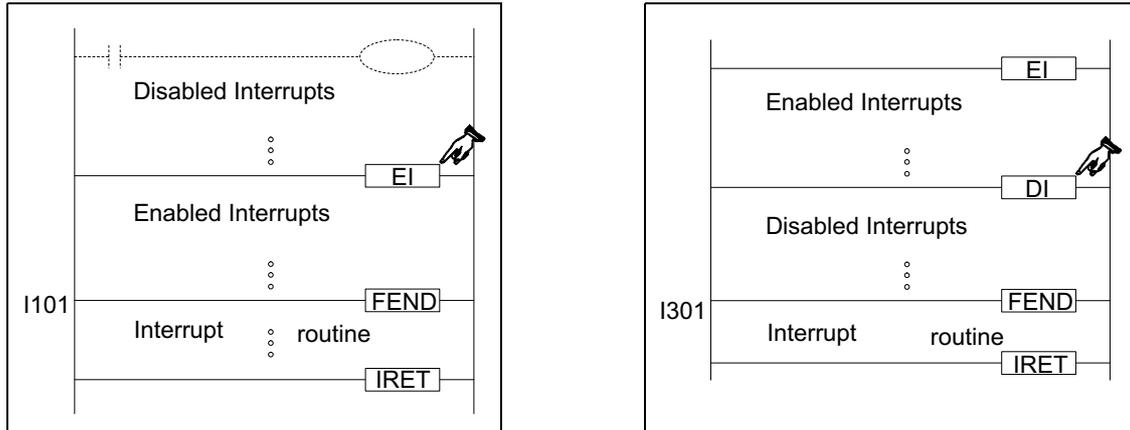
If an individual interrupt is to be disabled its associated special M coil must be driven ON. While this coil is ON the interrupt routine will not be activated. For details about the disabling M coils see the PLC device tables in chapter 8.
