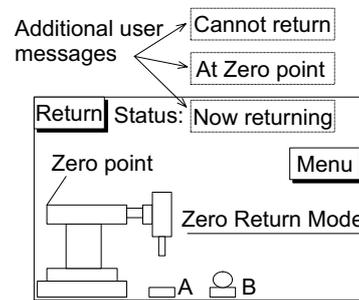
Once the zero point has been returned to, the operator would also return to the mode selection screen. This is achieved by pressing the 'Menu' touch key. This then resets the zero return bit device M31 which allows the DU screen change to take place.
