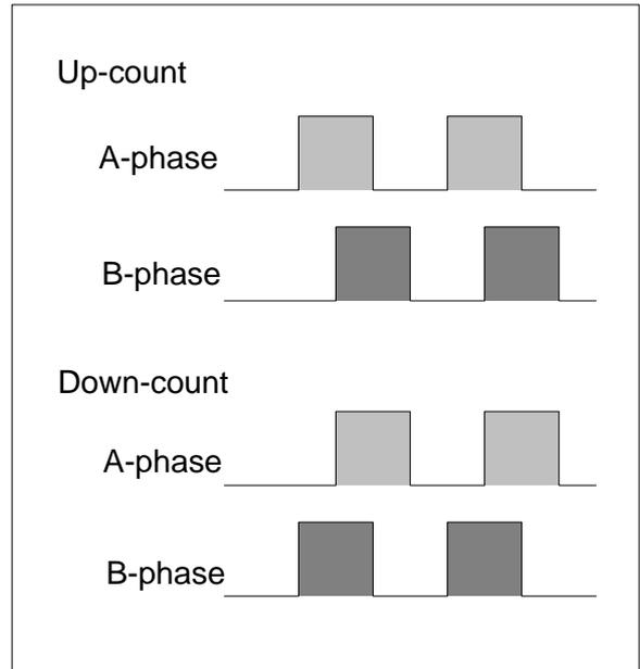
C251 counts the ON/OFF events of input X0 (the A phase input) and input X1 (the B phase input) while X11 is ON.
