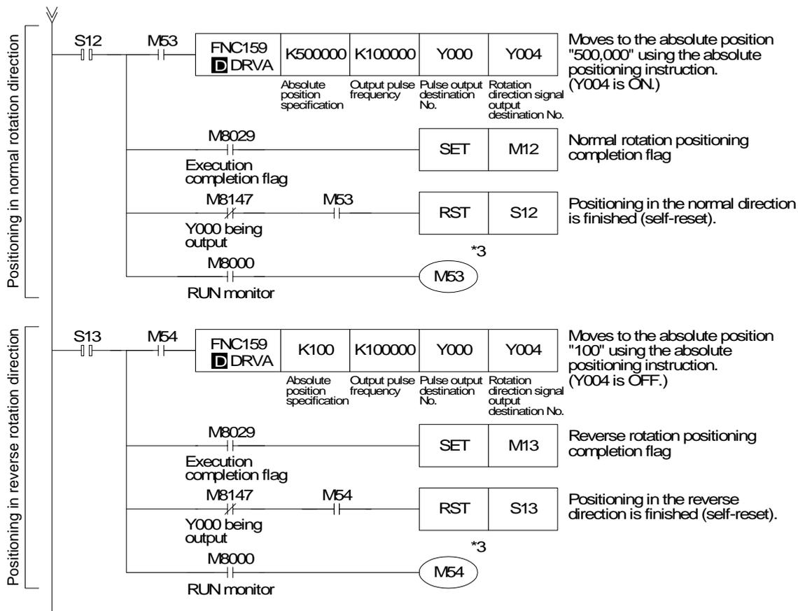
\*3 The instruction drive timing is delayed by one operation cycle to prevent simultaneous driving of positioning instructions.
