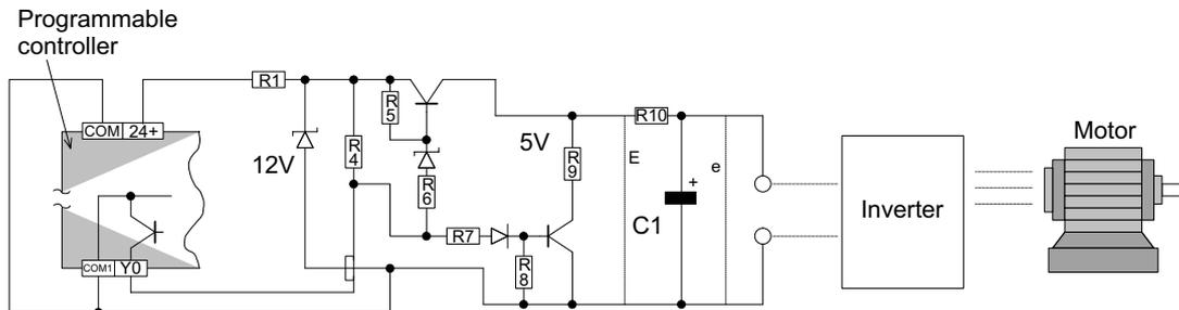
Circuit configuration for a PLC with sink outputs.
