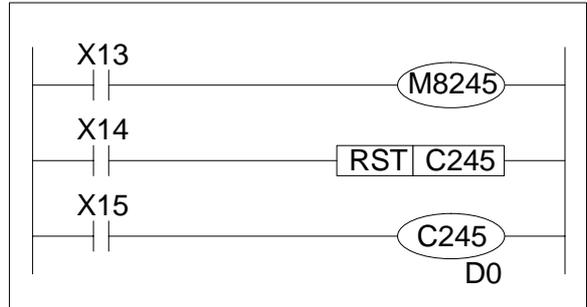
Counter C245 also has an external start contact, again automatically assigned. This is actually input X7. Once again this data can be found on the previous counter tables.
