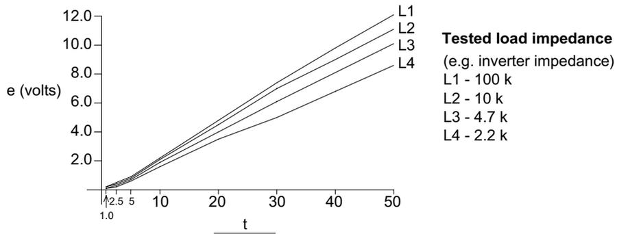
The duration of the  $T_0$ , time base also affects the ripple voltage. This can be clearly seen in the next set of test data:
