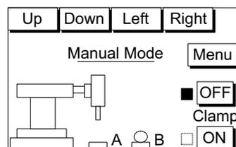
Once manual operation is completed the operator can return to the main mode selection screen by touching the 'Menu' key. This causes the manual mode bit flag, M30, to be reset. Once M30 is reset the DU screen then changes back to the desired mode selection screen.
