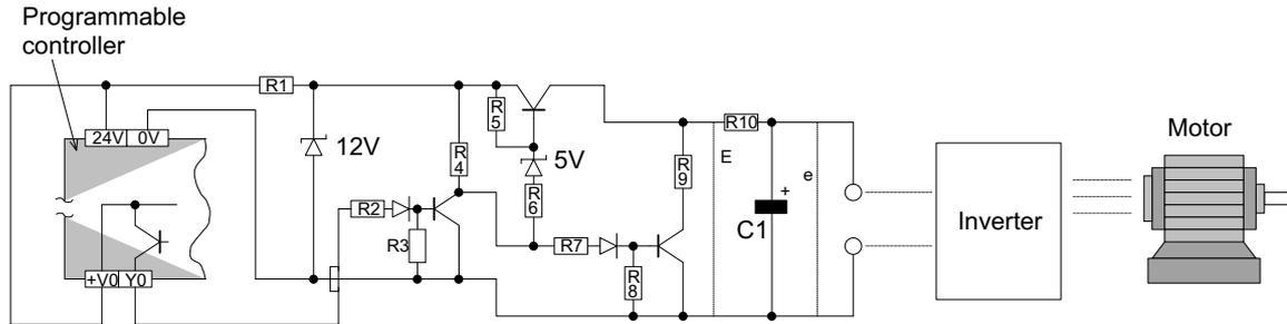
Circuit configuration for a PLC with source outputs
