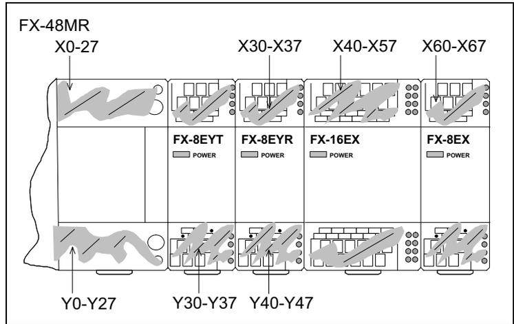
For easy use and identification, each additional I/O unit should be labeled with the appropriate I/O numbers using the provided number labels.
