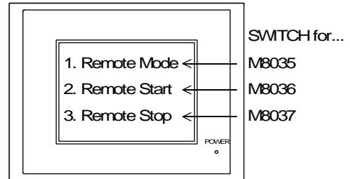
The HMI should be programmed with 'SWITCH' devices driving the three special M codes M8035,36 and 37. By activating the 'SWITCH' devices for M8035 and M8036 the PLC can be switched into a RUN state, while driving the 'SWITCH' device M8037 will put the PLC into a STOP state.
