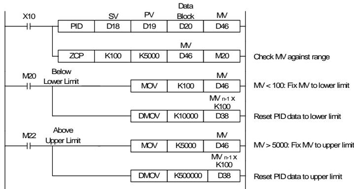
If data registers are used to hold the limit values, it is possible to use a MUL instruction instead of the DMOV. E.g. When D50 is upper limit use: MUL D50 K100 D38 because the result of MUL is already a double word DMUL is not needed.
