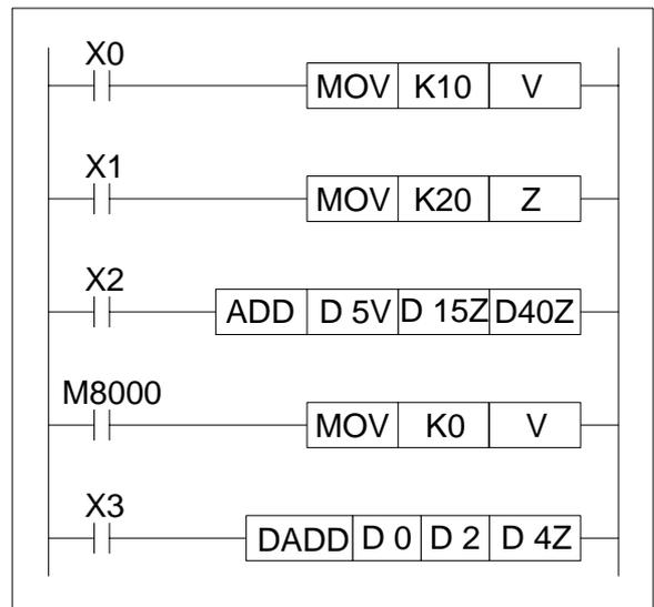
Both V and Z registers are initially set to K10 and K20 respectively.
