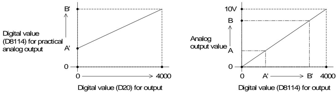
This example is equivalent to setting an offset and gain for the analog output.
