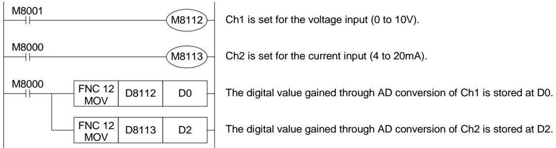
D0 ranges from 0 ~10000. To convert D0 to the 0 ~ 4000 value needed for D8114:
