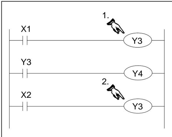
Double or dual coiling is not a recommended practice. Using multiple output coils of the same device can cause the program operation to become unreliable. The example program shown opposite identifies a double coil situation; there are two Y3 outputs. The following sequence of events will occur when inputs X1 = ON and X2 = OFF;
