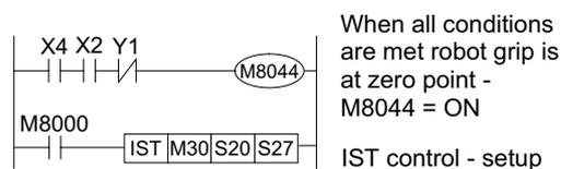
When the IST instruction is used there are 5 selectable modes which access three separate programs. This example has the following programs associated with its modes. Each mode is selected through the FX-40DU-TK. The screen shown opposite is the initial mode menu. Each of the menu options causes a screen jump to the selected mode. Menu options 1 and 3 also set ON auxiliary devices M30 and M31 respectively.
