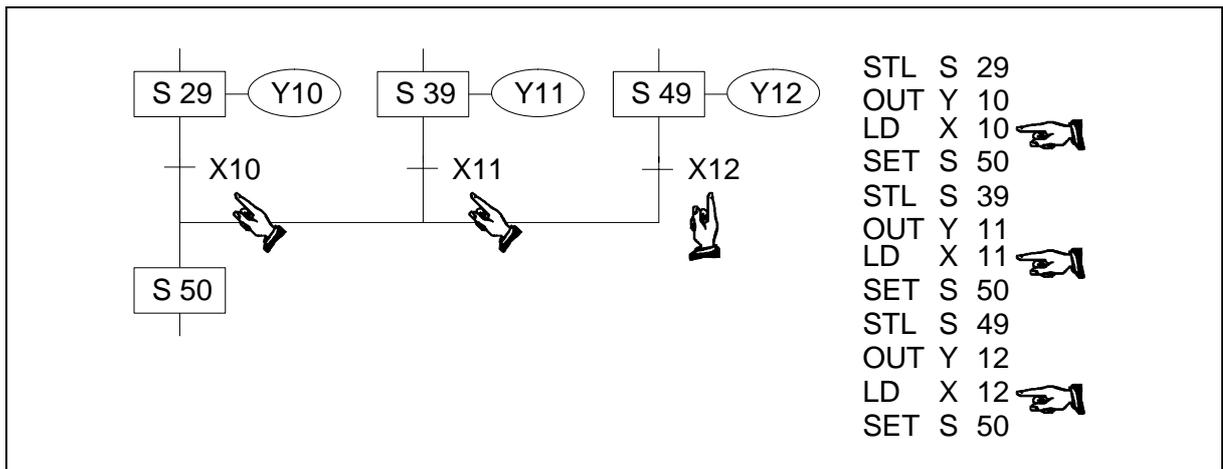
This type of STL program construction is called a "First State Merge" simply because the first state (in the example S29, S39 or S49) to complete its operation will cause the merging state (S50) to be activated. It should be noticed how each of the final STL states on the different program branches call the same "joining" STL state.
