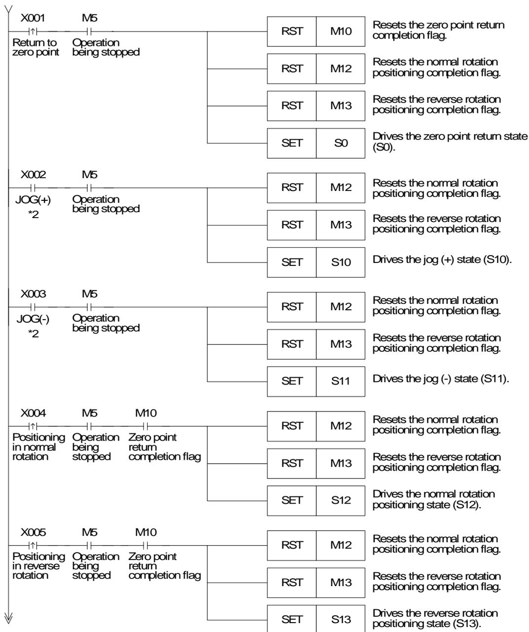
\*2 The maximum size of a JOG command is 999,999 pulses, as this is the maximum number of output pulses for a FNC 158 (DRVI) instruction. If a greater distance is required execute more than one JOG command.
