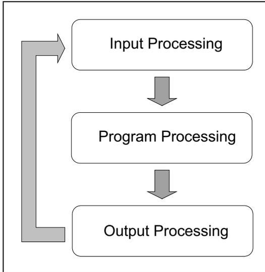
All of the current input statuses are read in to a temporary memory area; sometimes called an image memory. The PLC is now ready for the next program processing.....
