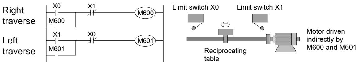
The status of the latched devices (in this example FX M coils M600 and M601) is retained during the power down. Once the power is restored the battery backed M coils latch themselves in again, i.e. the load M600 is used to drive M600.
