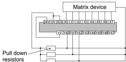
f) Because this instruction uses a series of multiplexed signals it requires a certain amount of 'hard wiring' to operate. The example wiring diagram to the right depicts the circuit used if the previous example instruction was programmed. As a general precaution to aid successful operation diodes should be placed after each input device (see diagram opposite). These should have a rating of 0.1A, 50V.
