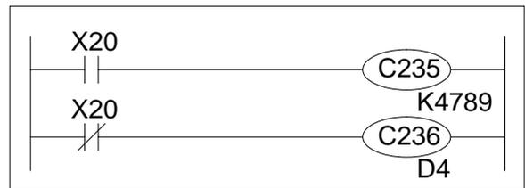
When X20 is OFF, coil C235 is turned OFF and coil C236 is turned ON. Counter C236 has an assigned input of X1, again the input X20 is NOT the counted input.
