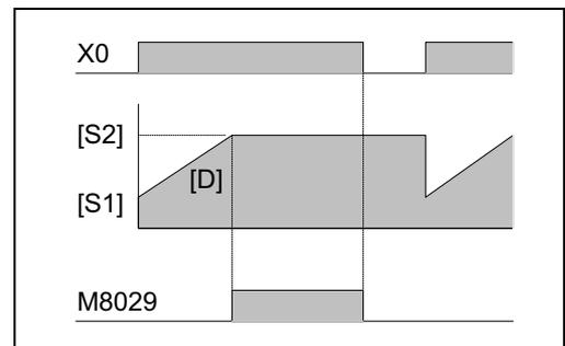
means once the current value of D equals that of S2, the RAMP instruction will 'freeze' in this state. This means the M8029 will be set ON for as long as the instruction remains energized and the value of D will not reset until the instruction is re-initialized, i.e. the RAMP instruction is turned from OFF to ON again.
