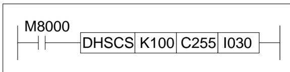
The sequence programmed after the label (indicated by the I030 pointer) is executed once the value of High Speed Counter C255 reaches/equals the preset limit of K100 identified in the example HSCS.
